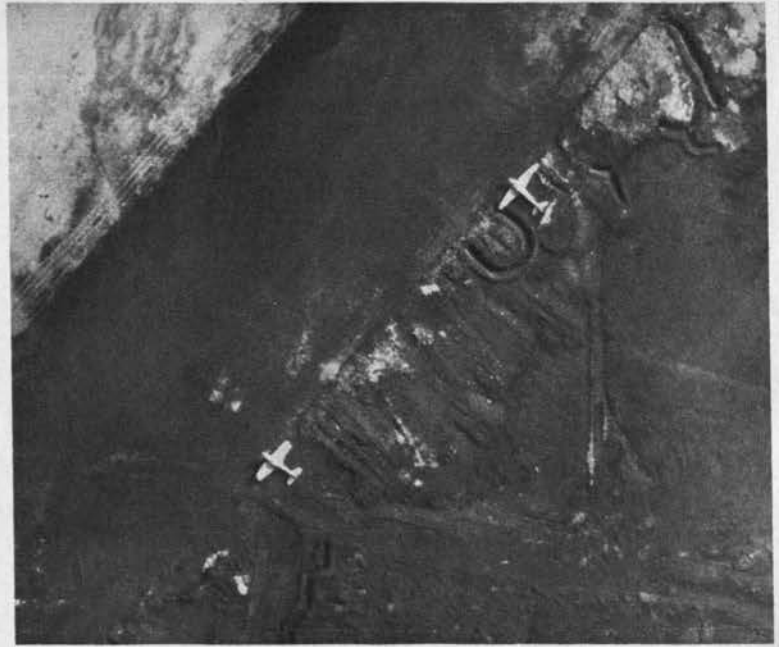
Additional dummies on the Ie Shima airfield can be spotted because of their freak wing shapes, failure to resemble known types of aircraft.
